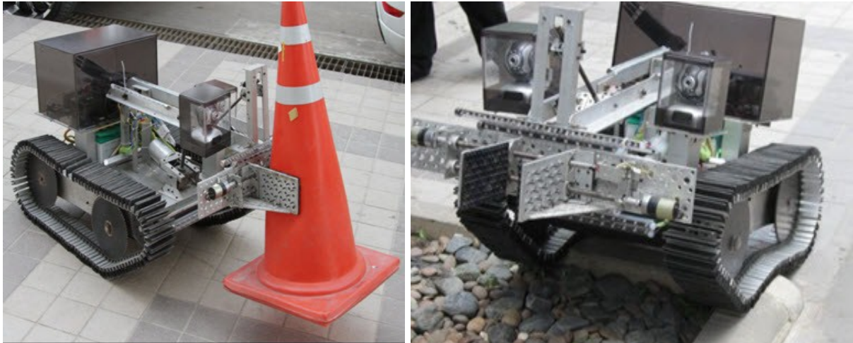
Figure 11 (left) displays the proposed robot v.2 carrying the object. Figure (right) shows the robot v.2 moving on the rough road.
