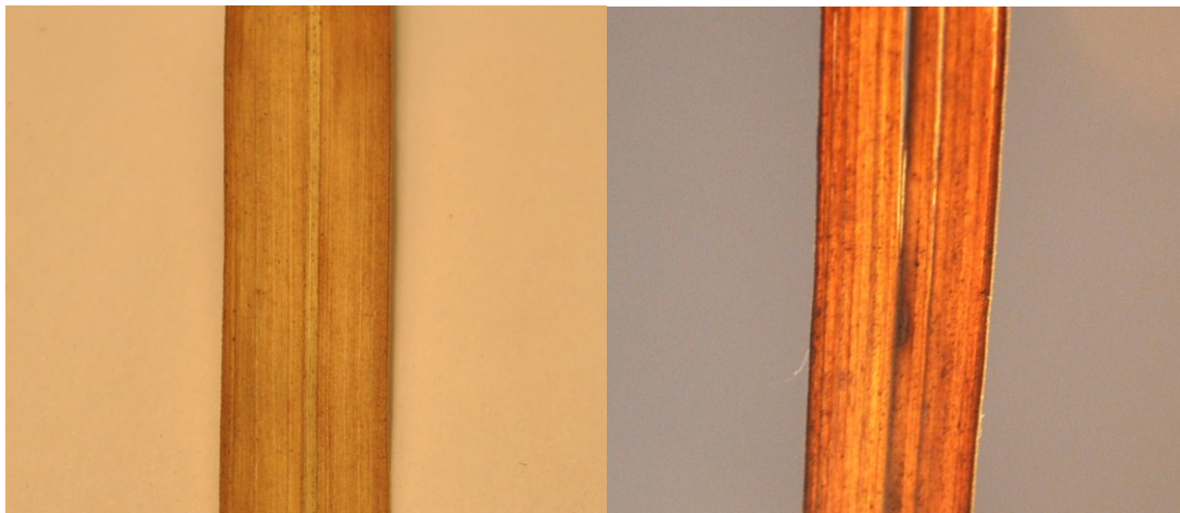
Figure 1 (Left) Show the reflectance of thatched grass blade. (Right) The lower side of thatched grass blade, it is translucent.
